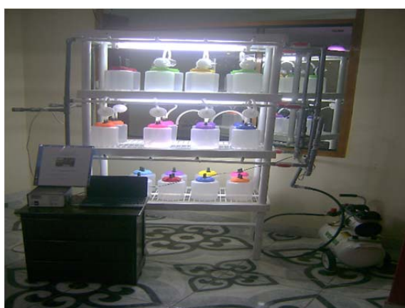
Fig. 1. Pneumatic temporary immersion bioreactor system assembled and its operation.
