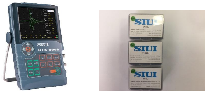
Figure 2. UT Inspection Device and Probes
